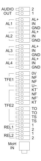
Supply Voltage for Sensor 1 Signalling Input Sensor 1 Ground Supply Voltage for Sensor 2 Ground Supply Voltage for Sensor 3
