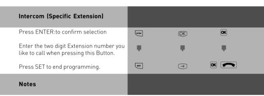
If you assign the Extension of a Telephone Answering Machine, then you can Pick Up the call even after the Machine has answered it. This is providing that the Port is set to Answering machine. If no extension has been set on the Intercom Button, then you can dial any extension after this Button has been pressed.
