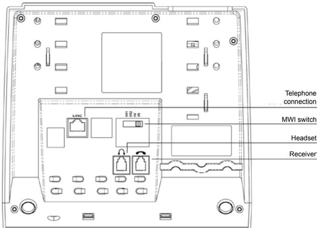
The MWI (Message Waiting Indicator) switch is for switching between the various message displays of a PBX.
