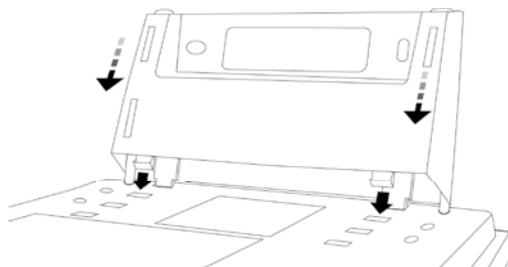
For wall mounting, fit the unit stand to the wall using two screws as shown (Fig. 1). Then fit the phone to the unit stand (Fig. 2). Take out the plastic component in the receiver cradle, turn it through 180 degrees and reinsert (Fig. 3).
